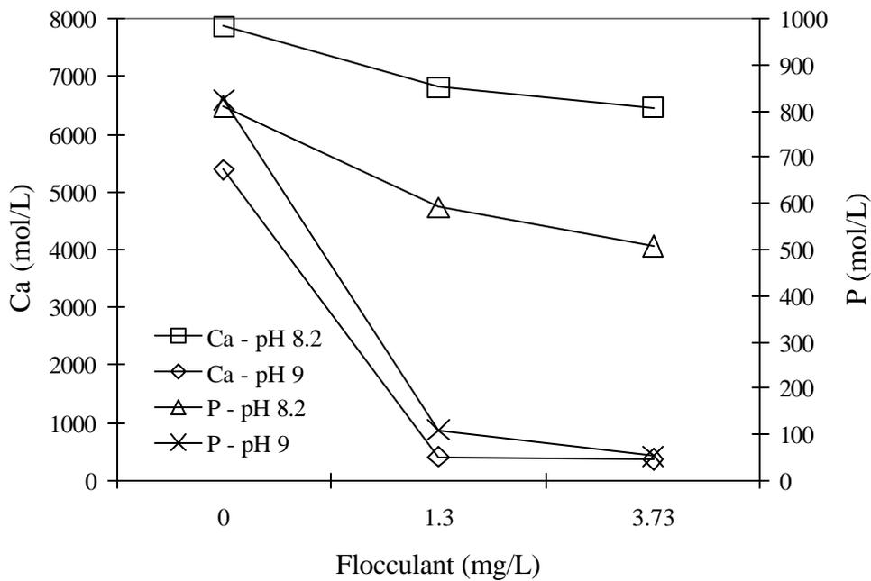
Figure 3: Calcium (Ca) and phosphorus (P) concentrations with pH changes over different flocculant concentrations
