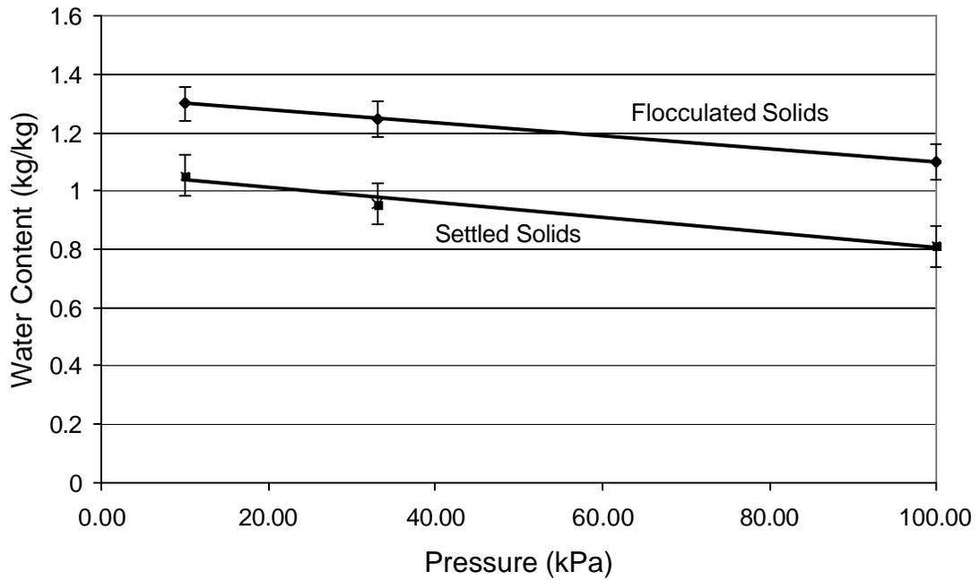
Figure 4: Water holding capacity of the flocculated and settled solids
