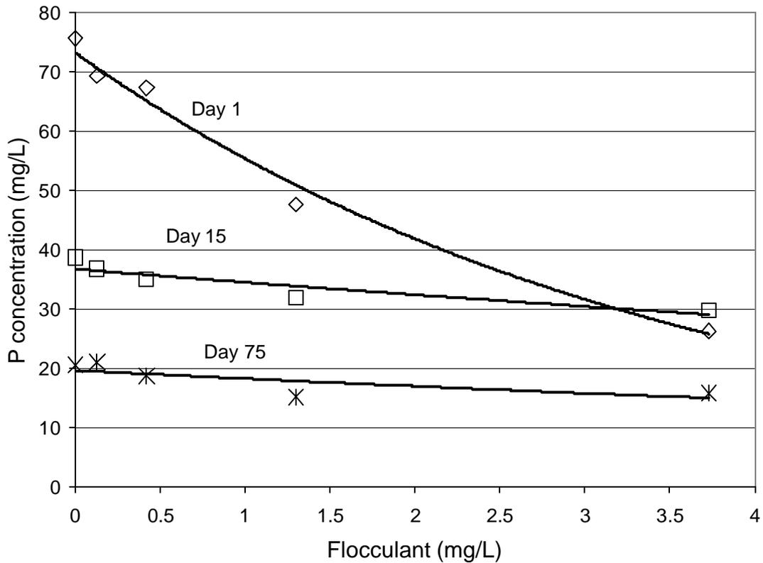
Figure 2: Changes in phosphorus (P) with increasing flocculant added to effluent wastewater.
