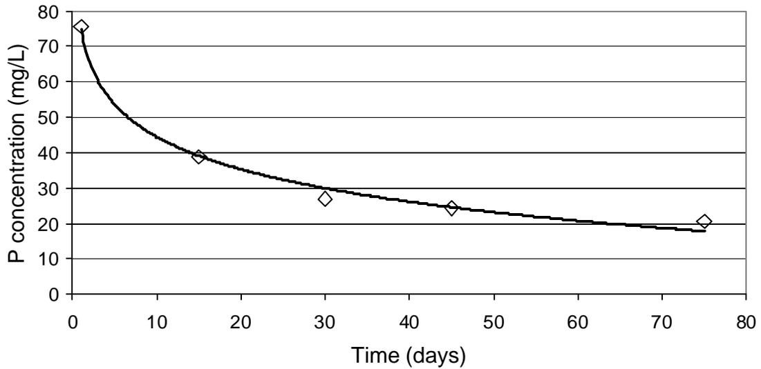
Figure 1: Changes in phosphorus (P) concentration caused by settling of suspended solids over time.
